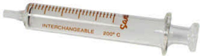
**Note:** While operating a biodiesel processor, you are almost certain to get waste vegetable oil or biodiesel on your hands and fingers. If this oil is transferred to the printed numbers and line marking on a syringe, the printed marks will dissolve and smear to become illegible. I have not found a plastic syringe that is impervious to biodiesel or waste vegetable oil but almost all glass syringes are.
