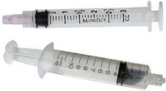
**Note:** Do not attempt to suck up biodiesel into a plastic syringe. Biodiesel will destroy the black rubber tip of the plunger the very first time it contacts it. While titrations do not require any biodiesel sampling, quality testing does. I strongly recommend surfing Ebay for a quality two piece glass syringe in the 5ml to 10ml size range.
