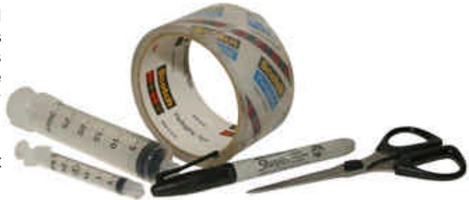
To solve the oily fingers problem, the best solution I have found is to wrap the outside of the syringe with normal clear packing tape. If you wrap it neatly in sections, you will never even see the tape on the syringe. You should also label each syringe for its purpose and use the syringe only for that purpose.
